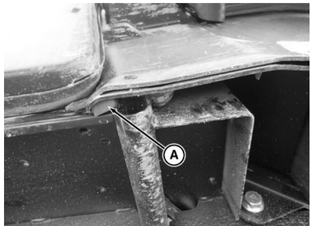
View of bottom of B-pillar cover looking up
